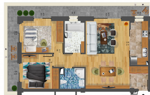
Apartment 14 Etaj 3 Sufragerie = 26.80mp Bucatarie = 5.95mp Hol = 3.20mp Buc = 4.40mp Grup Sanitar = 3.75mp Camera = 10.50mp Biro = 9.45mp Suprafata Utila = 64.50mp Terasa = 17.55mp Suprafata = 82.05mp
